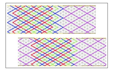
IT IS POSSIBLE to have "distant" NESTED-BIGHT by putting LEFT BIGHT RIM 2 farther from LEFT BIGHT-RIM 1 while retaining the distance between BIGHT RIM 2 AND 3 (if you do not comply with that the half-period coding will be faulty when using PINAPL or PINAPL2 as they are.
