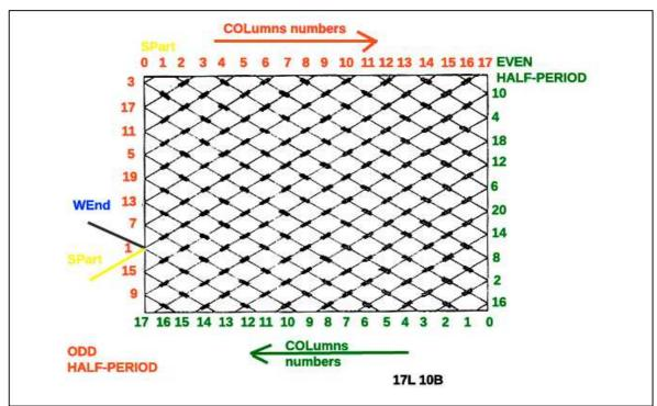
**FIRST: PREPARE THE DIAGRAM.** Here HORIZONTAL MANDREL FRAME of REFERENCE. Just make an anti-clockwise rotation of Pi/2 or 90° to get the vertical cylinder frame of reference.
